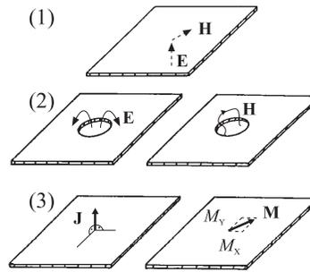
Fig. 10.4: Explanation of the hole coupling
