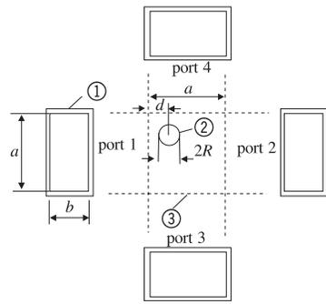
Fig. 10.5: Cross coupler with a circular coupling hole with a diameter of  $2R$
