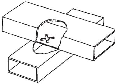
Fig. 10.3: Principal design of a waveguide (cross directional) coupler and including port numbering
