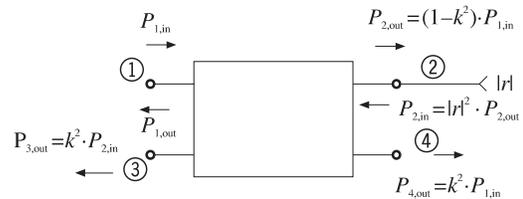
Fig. 10.2: Use of the directional coupler as a reflectometer
