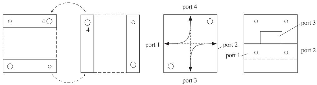
Fig. 10.9: On the numbering of the ports of the cross-coupler (here, for example, port 4 is marked)
