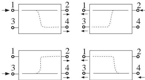
Fig. 10.1: Principal response of a directional coupler
