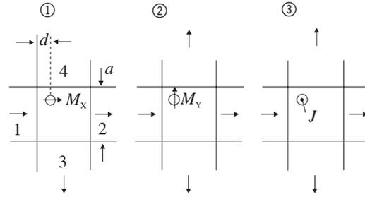
Fig. 10.6: Wave excitation when feeding wave into port 1
