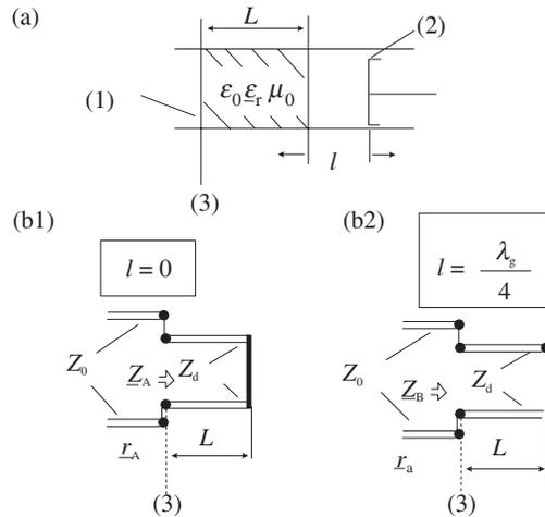
Fig. 9.1: (a) Measurement configuration with material sample (1) with the length  $L$  and moveable short (2) connected downstream. Distance of the short-circuit plane from rear side of material sample is  $l$ . Reference plane for measurement is (3). (b) Equivalent circuit diagram for trans. line for computation of the input impedances  $Z_A$  and  $Z_B$  for the short-circuit ( $l=0$ ) and open-circuit case ( $l = \lambda_g/4$ ).
