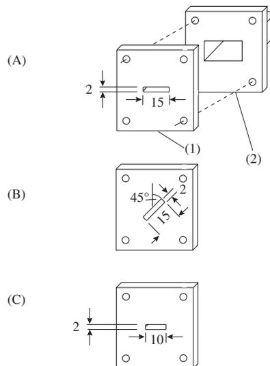
Fig. 8.3: Dimensions and alignment of the three slot antennas used here
