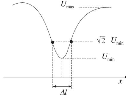
Fig. 6.2: For the determination of  $s$  and  $|r|$  from the measurement of the “node width”  $\Delta l$ .
