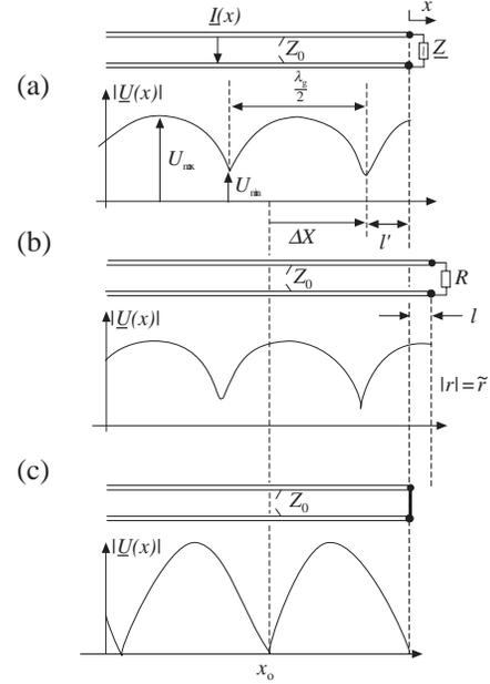
Fig. 6.1: Voltage distribution along a transmission line
