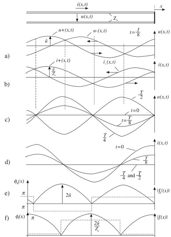
Fig. 5.3: Standing wave on a line shorted on one end:
