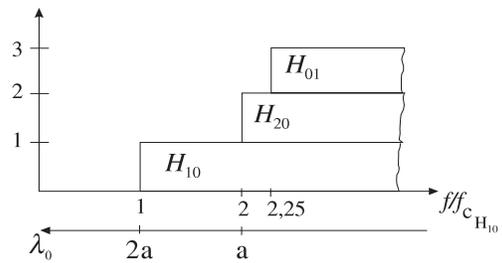
Fig. 5.6: Existence zones for various wavetypes capable of propagating in the rectangular waveguide ( $a = 2.25 b$ ).
