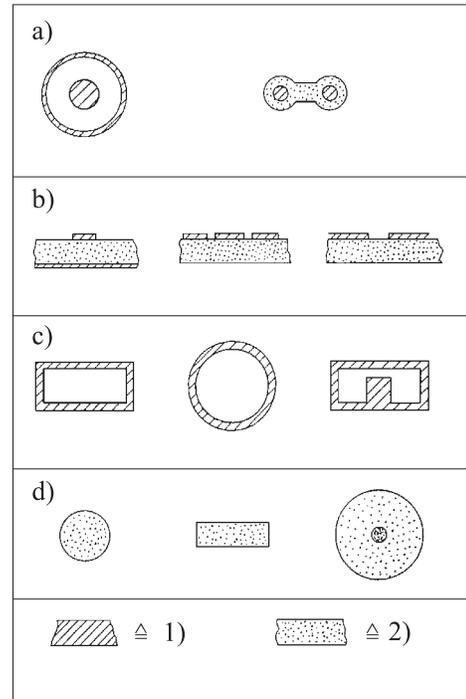
Fig. 5.1: Various line types for electromagnetic waves (1 = metal conductor, 2 = isolator). Numbering from left to right.
