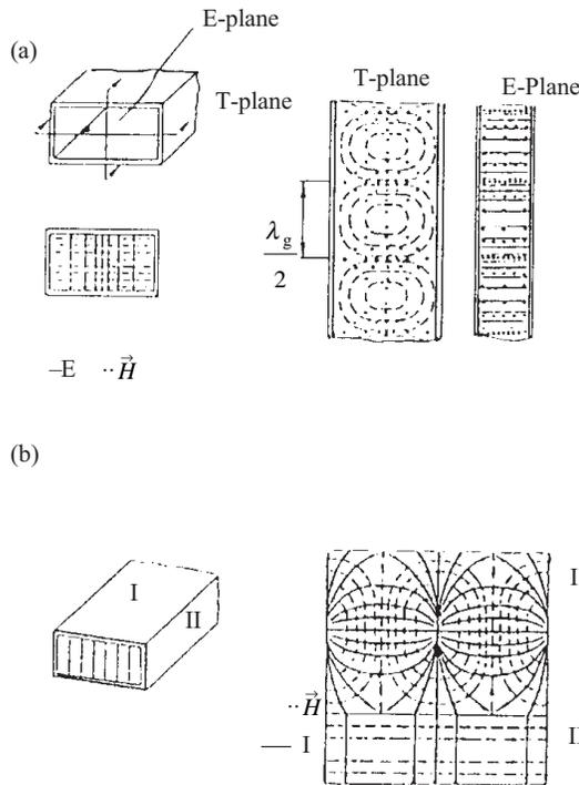
Fig. 5.5: Field pattern of the fundamental mode ( $TE_{10}$ -wave) in the rectangular waveguide
