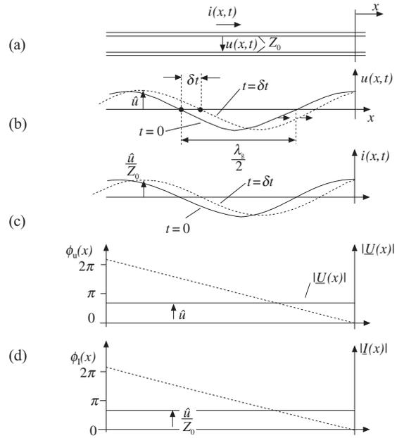
Fig. 5.2: Wave propagation on a line
