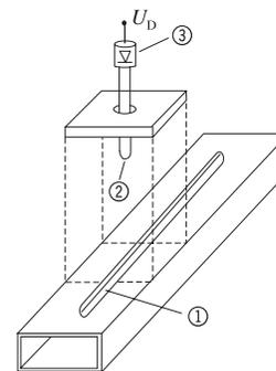
Fig. 5.7: Principle of the slotted measuring line (exploded view)
