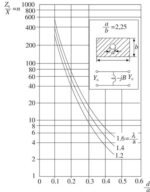
Fig. 12.4: Normalized transformation ratio for the coupling diaphragm  $Z_0/X$ .  $\lambda$  corresponds here to the free-space wavelength  $\lambda_0$
