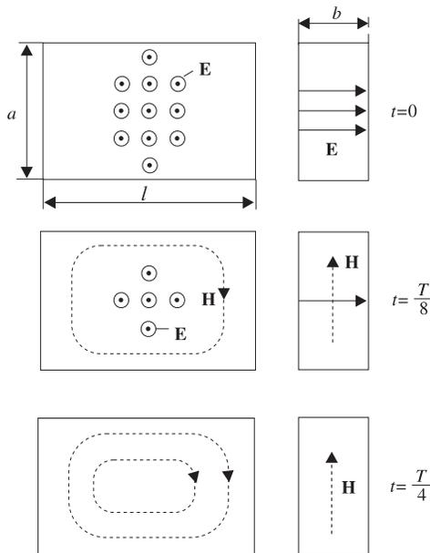
Fig. 12.1:  $TE_{101}$  resonance in a rectangular cavity resonator
