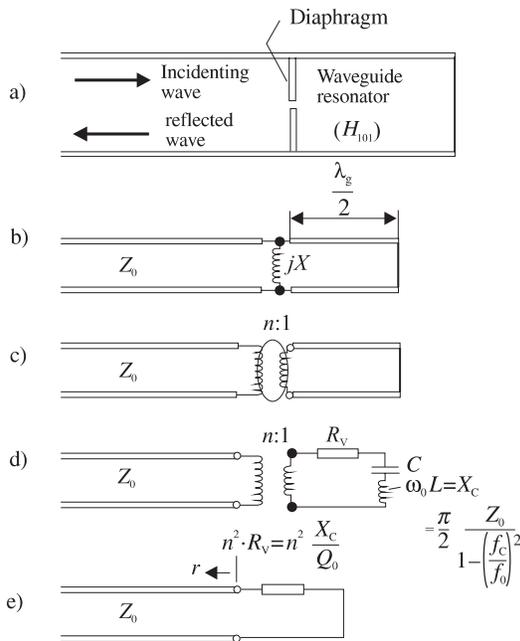
Fig. 12.3: Development of an equivalent circuit diagram for the cavity resonator coupled via a diaphragm with aperture
