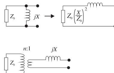
Fig. 12.2: Series equivalent circuit diagram for resonators with coupling diaphragm
