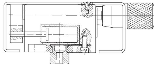
Fig. 4.2: Cross-section through the attenuator 737 09
