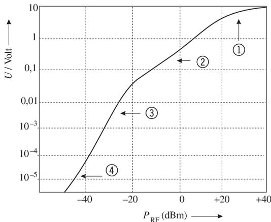
Fig. 4.3: Detector output voltage as a function of the microwave power
