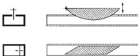
Fig. 4.1: On the principle of attenuation by means of insertion with an attenuating vane
