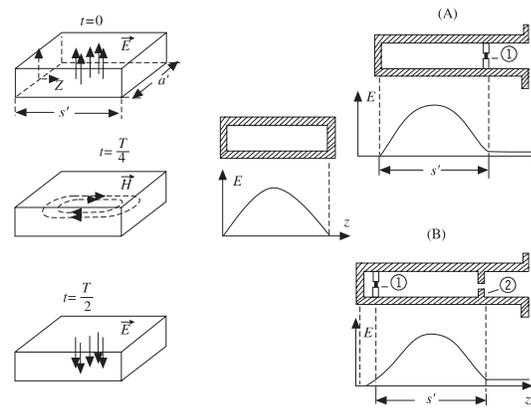
Fig. 1.2: Basic design of the Gunn oscillator
