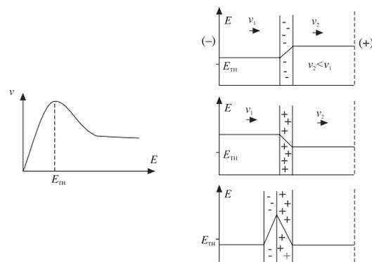
Fig. 1.1 Principle of a Gunn diode
