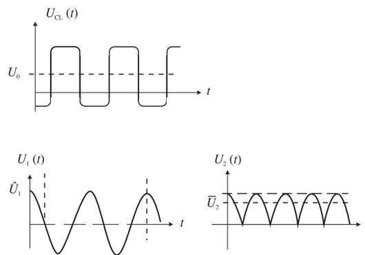
Fig. 3.5: Voltage characteristics of the single phase-sensitive rectifier
