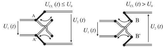
Fig. 3.4: Voltage controlled switch as phase-sensitive rectifier (PSD). Switch set to position A, if voltage  $U_{cl}(t)$  of clock generator is smaller than threshold value  $U_0$ . Otherwise in setting B.
