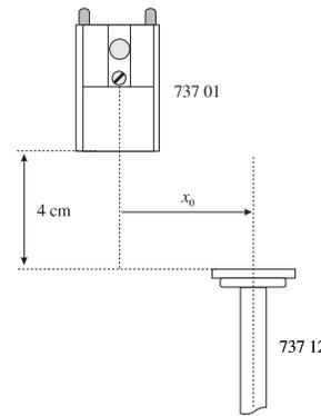
Fig. 3.7: Transverse shift of the waveguide axes (view from above)
