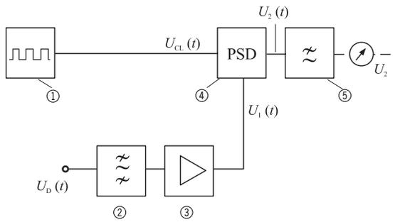
Fig. 3.3 Design of the lock-in amplifier
