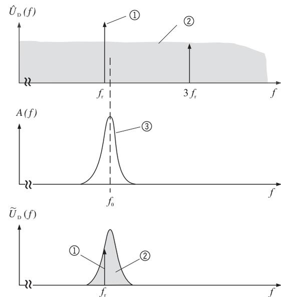
Fig. 3.2: Frequency spectrum of the signals according to Fig. 3.1 upstream (above) and downstream (below) from a narrow-band bandpass filter.
