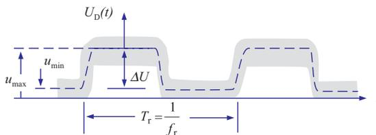
Fig. 3.1: Dynamic characteristic of the output signal of the E-field probe with superpositioned noise voltage ( $f_r = 976$  Hz)
